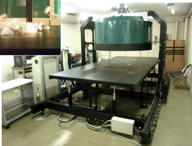
Photo 4. The BRI's tornado simulator
