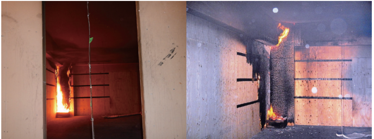
Photo 5: Fire behavior in wooden interior finish spaces (left, when heated at 100 kW; right, at the end of the test)
