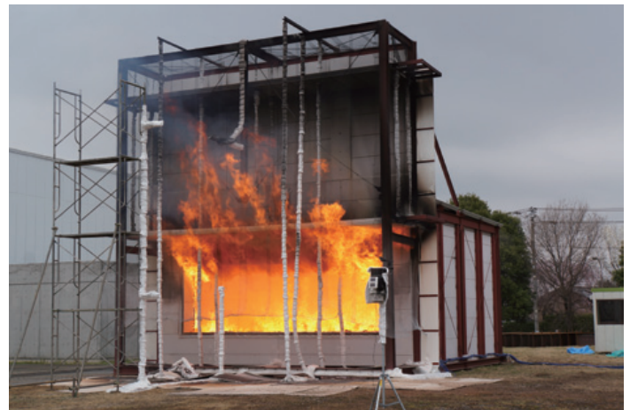
Photo 6: Fire test using classroom-sized compartment
