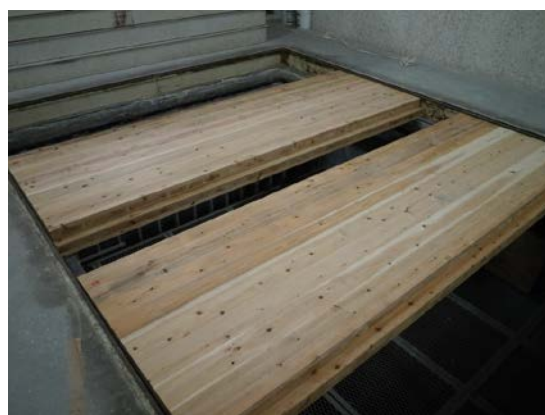
Right: Interior of reverberation room - experiment of timber floor
