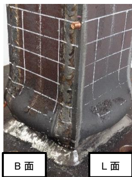
(i) B-L 面柱脚部詳細
