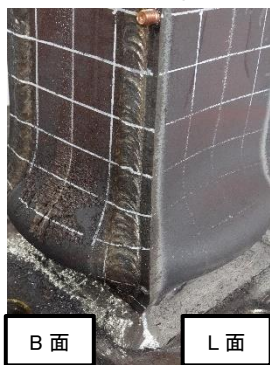
(i) B-L 面柱脚部詳細
