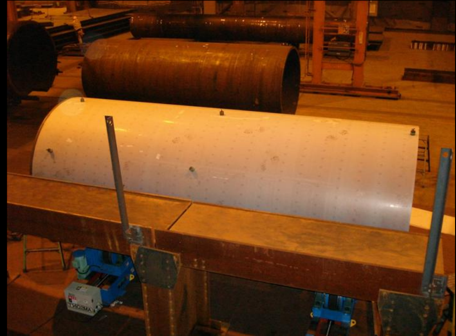
Confirm the position of 700+ studs
